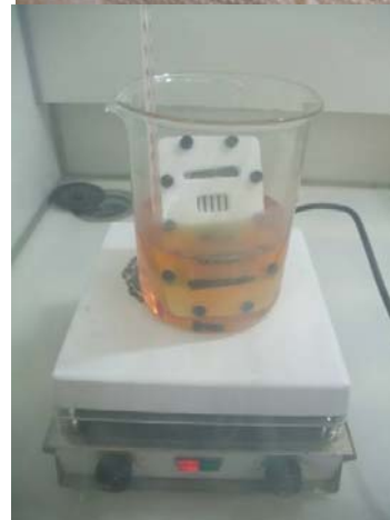
Fig.1. the etching experimental setup.
