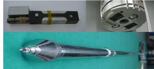
Figure 8. Specimen, Al holder and capsule
