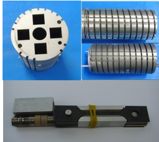
Figure 4. Al holder (thermal media) and ring/plate tensile specimen
