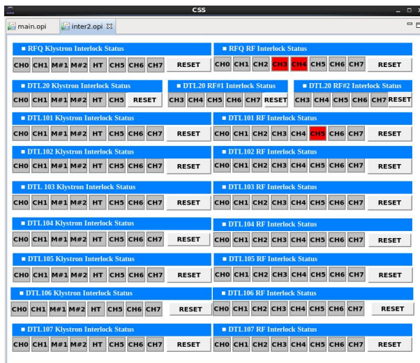
Fig. 3 Graphic User Interface (GUI) for monitoring operating status of RF and klystron interlock system
