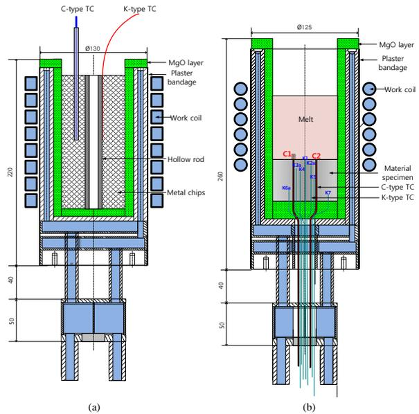
Fig. 6. Configurations of the cold crucibles; (a) melt crucible, (b) interaction crucible
