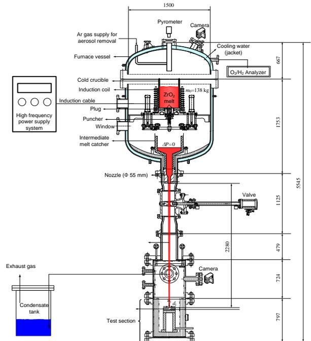
Fig. 2. A schematic of VESTA facility
