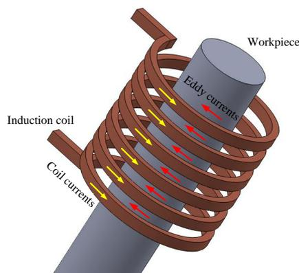
Fig. 1. A conventional induction heating system
