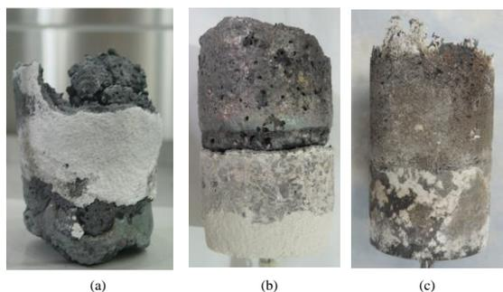
Fig. 7. Metal ingot and material specimens; (a) metallic corium melt-concrete, (b) stainless steel melt-concrete, (c) stainless steel melt-Inconel 690
