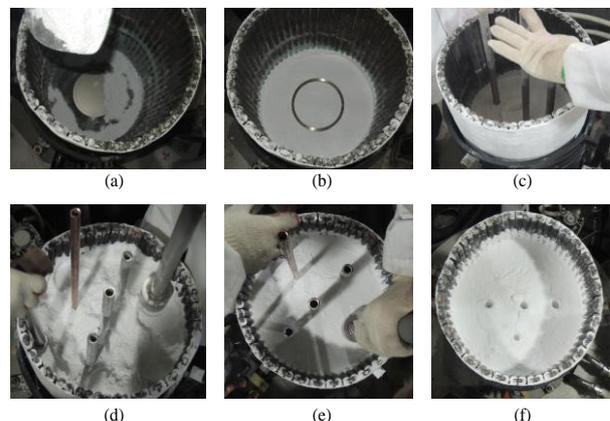
Fig. 3. ZrO<sub>2</sub> power filling process in a cold crucible
