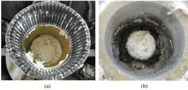
Fig. 4. Images after the experiment; (a) cold crucible, (b) concrete specimen in the test section
