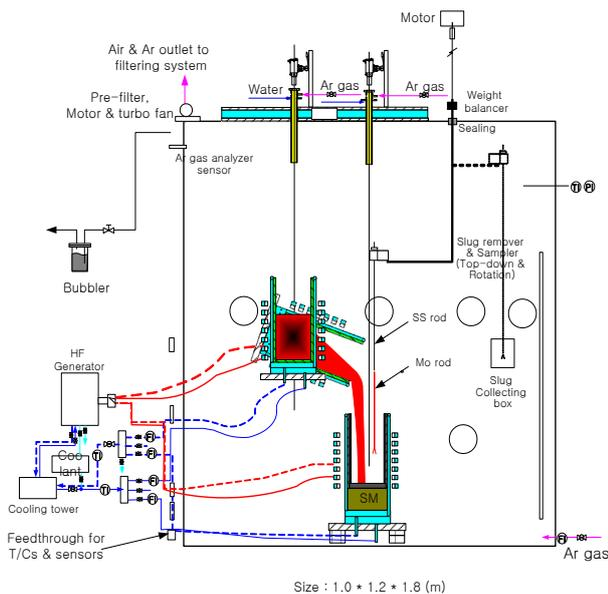
Fig. 5. A schematic of VESTA-S facility
