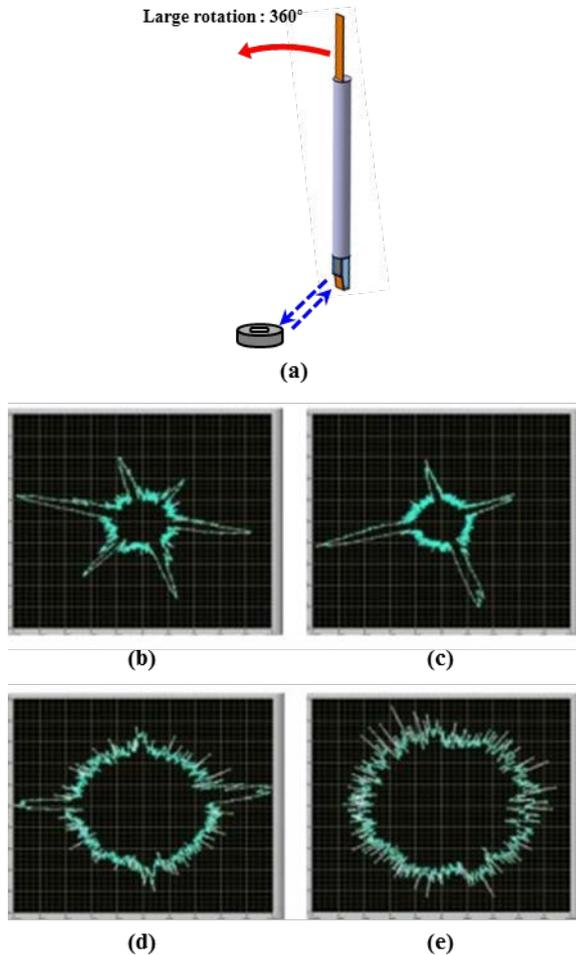
Fig. 4. (a) Experimental setup for identification inspection. Radiation patterns of reflected waves from (b) hexagon nut, (c) square block, (d) pin and (e) washer.
