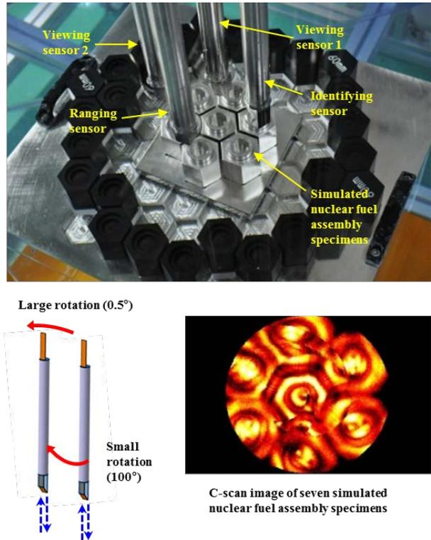
Fig. 3. Experimental setup and resulting image of viewing inspection.
