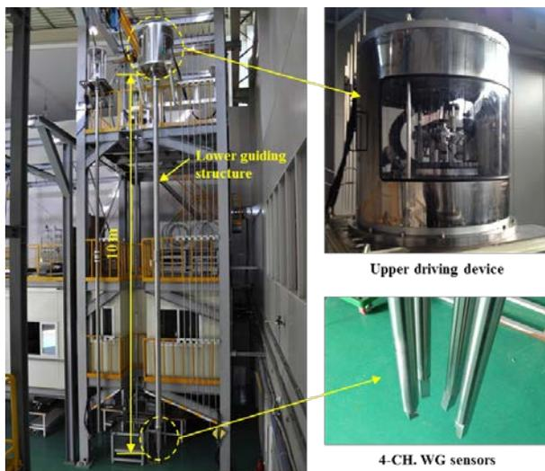
Fig. 1. The developed remote inspection module
