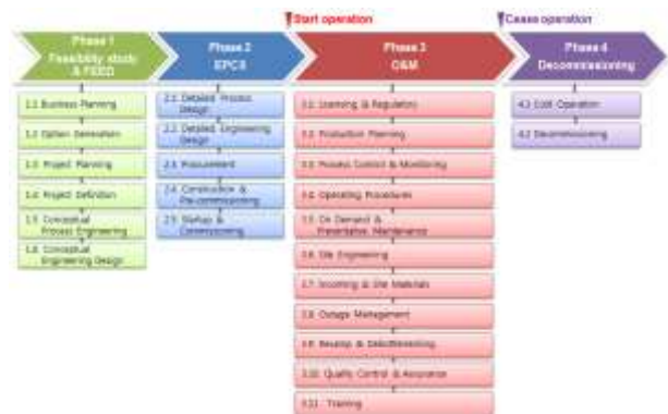
Fig. 1. Life cycle stage of nuclear power plant.
