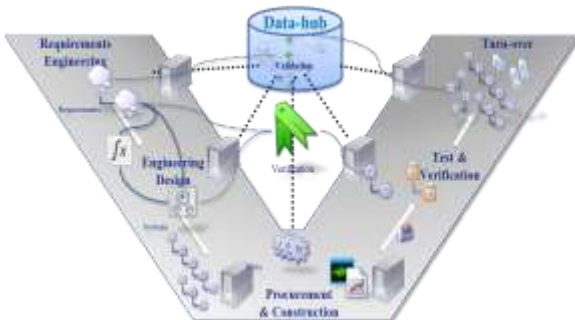
Fig. 4. V-Model based data centric CM concept for key relationship through life cycle perspective.
