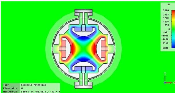
Fig.4. Potential distribution in the quadrupole.
