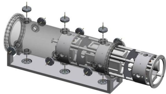
Fig.7. Electrostatic quadrupole triplet.
