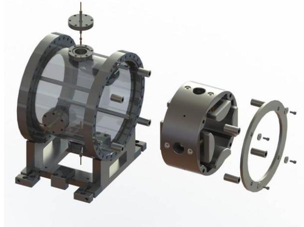
Fig.6. Electrostatic quadrupole singlet.
