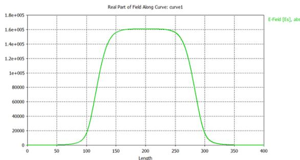
Fig.5. Magnitude of the electric field along beam axis.
