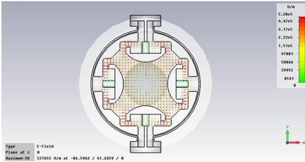
Fig.3. Electric field distribution in the quadrupole.
