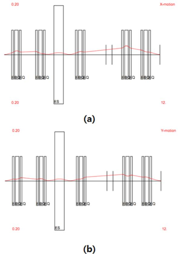
Fig.1. Beam envelop from HRMS to ECR charge breeder; (a) x plane envelop, (b) y-plane envelop.
