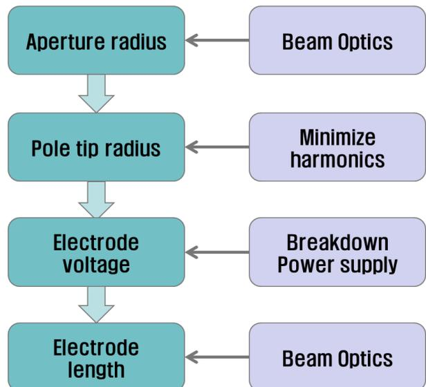
Fig.2. Design flow for ESQ parameters.
