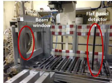
Fig. 2. Installation of FPD for proton beam irradiation
