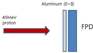
Fig. 4. The beam energy adjustment by aluminum plates
