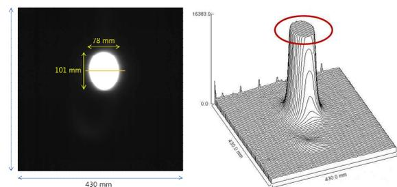
Fig. 3. The first obtained image and profile of proton beam
