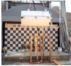
Fig. 4. Drop test from tip-over condition
