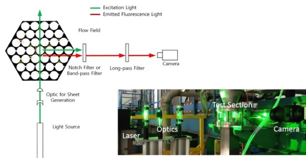
Fig. 2. Experimental configuration for LIF measurement
