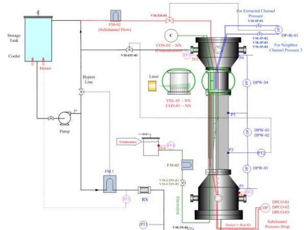
Fig. 1. FIFFA test loop diagram
