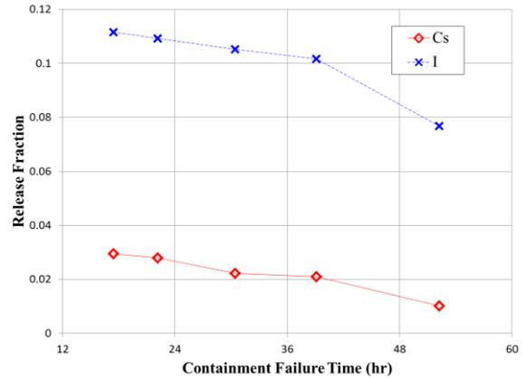
(b) release fraction vs. containment failure time
