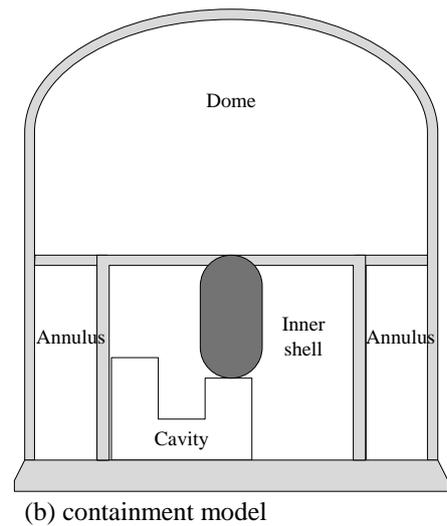
Fig. 2. A nodalization diagram of the reference plant
