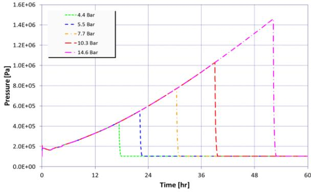
(a) effect of containment failure pressure
