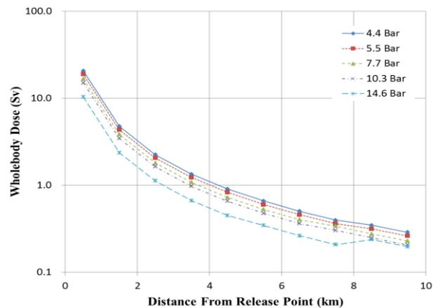
**Fig. 8. The relative peak wholebody dose for the containment failure pressure (except the failure time)**
