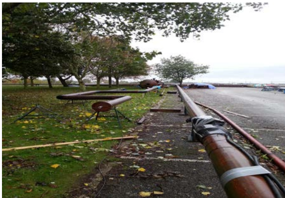
Fig. 1. Long range pipeline inspection specimen
