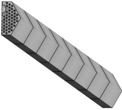
Fig. 1. CFD mesh for RSC fuel assembly
