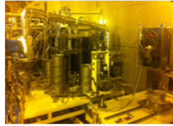
Fig.1 A Pride salt transport system in an Ar cell
