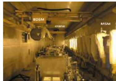
Fig.2. Remotely control tools within Ar Cell
