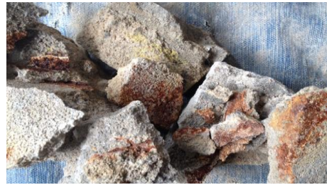
Fig. 1. The surface of a brick generated from the wall of a laboratory. A high concentration of uranium was found in the yellow or brown colored areas.
