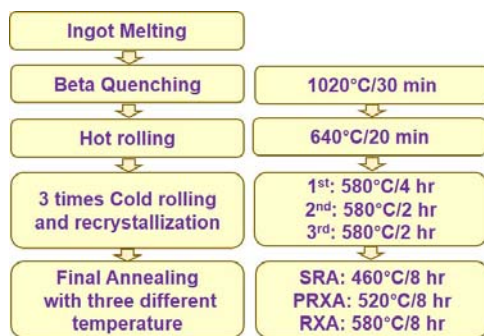
Fig 1. The manufacturing process of Zr-Nb-X experimental alloys
