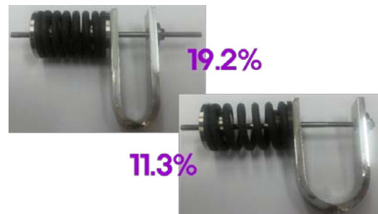
Fig. 1. Spring-loaded U-bend specimen for PWSCC initiation test
