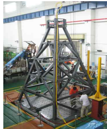
Fig. 1. Mounting of CEDM specimen with jig structure
