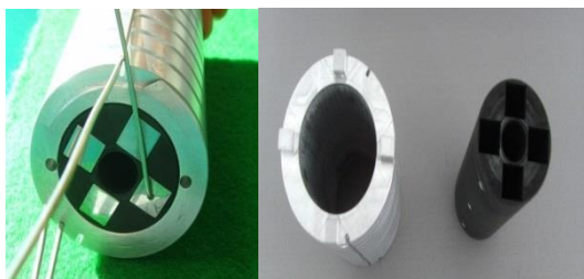
Figure 3. Structure of double thermal media
