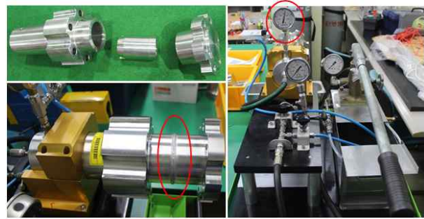
Fig. 6. Hydraulic pressure test of the EB welded part
