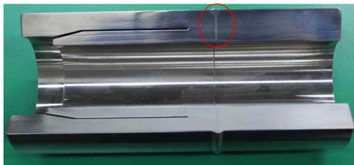
Fig. 5. Cross section of the EB welded part
