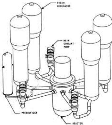
Fig. 1. Westinghouse 4-loop NSSS
