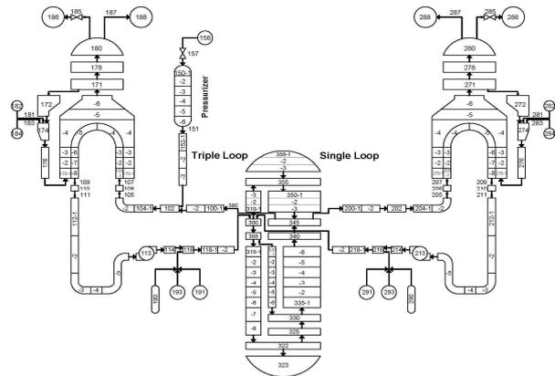
Fig. 2. Nodalization for the Zion unit 1 PWR
