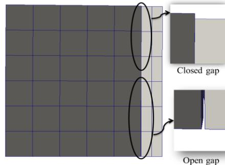
Fig. 3 Open gap region and closed gap region between pellet and cladding
