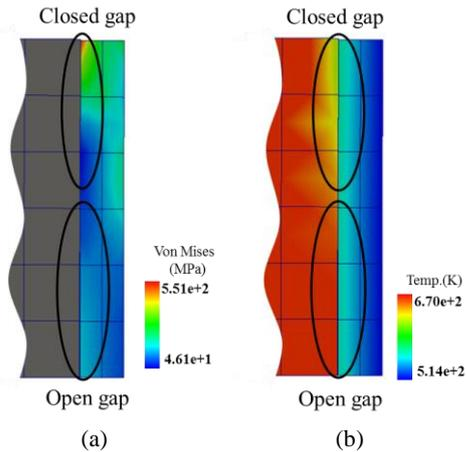
Fig. 4 (a) Von-Mises stress of the cladding and
