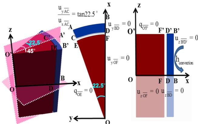
Fig. 2 (a) Boundary condition of the pellet and the cladding
