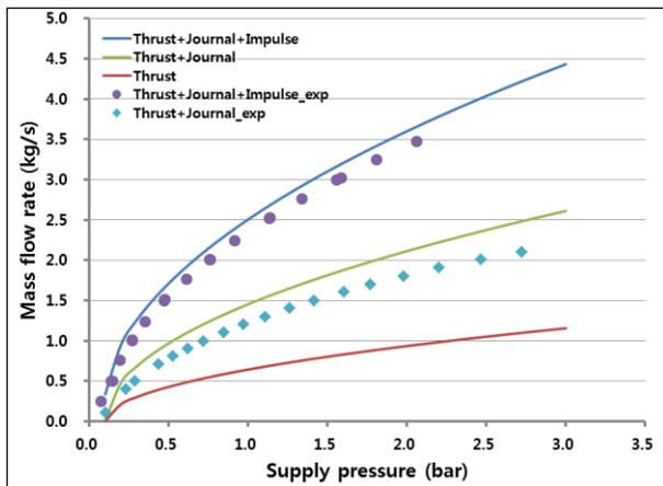
Fig. 3. Mass flow rate at the each nozzle (thrust bearing, journal bearing, and impulse jet).
