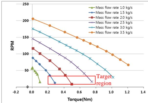
Fig. 6. RPM of the NTDHRD as a function of the torque at the constant mass flow rate.
