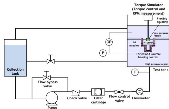
Fig. 2. Schematic of the experimental apparatus for the tests of NTDHRD.
