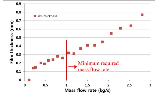
Fig. 4. Film thickness of the NTDHRD as a function of mass flow rate.
