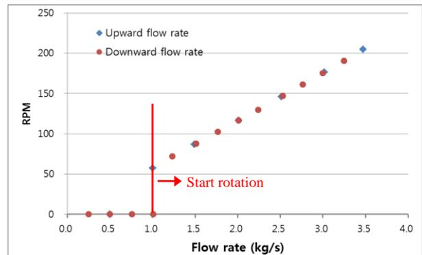
Fig.5. RPM of the NTDHRD as a function of mass flow rate.
