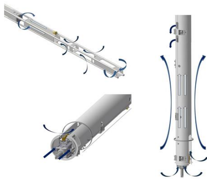
Fig. 4. Expected flow path around MAST assembly
