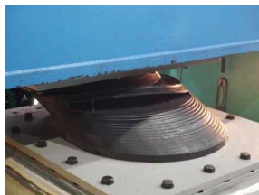
(b) failure after 2-D test (c) failure after 1-D test Figure 5. Deformed and failure shape of after 1-D, 2-D test
