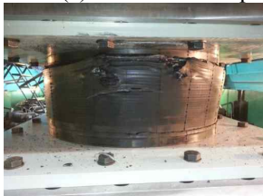
(b) failure after 2-D test (c) failure after 1-D test Figure 5. Deformed and failure shape of after 1-D, 2-D test
