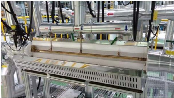
Fig. 3. Equipped plugging specimen for the sodium- $\text{CO}_2$  interaction test.
