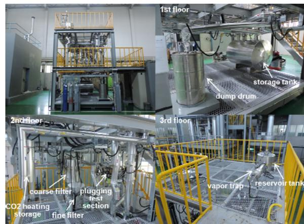
Fig. 2. Facility for the sodium-CO<sub>2</sub> interaction test.
