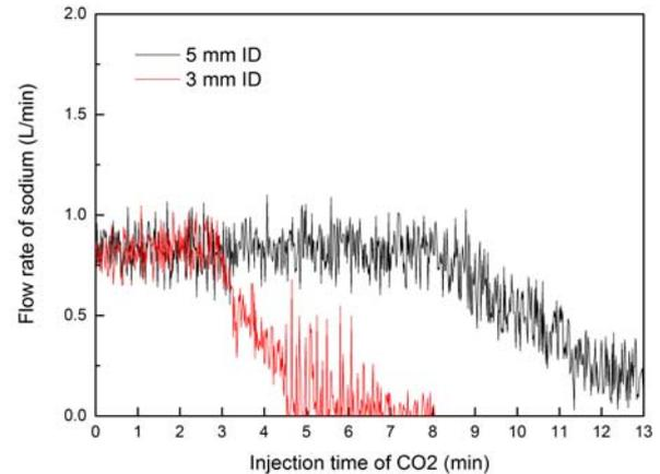
Fig. 4. Flow rates of sodium with 3 and 5 mm ID of sodium channels at 300  $^\circ\text{C}$ .
