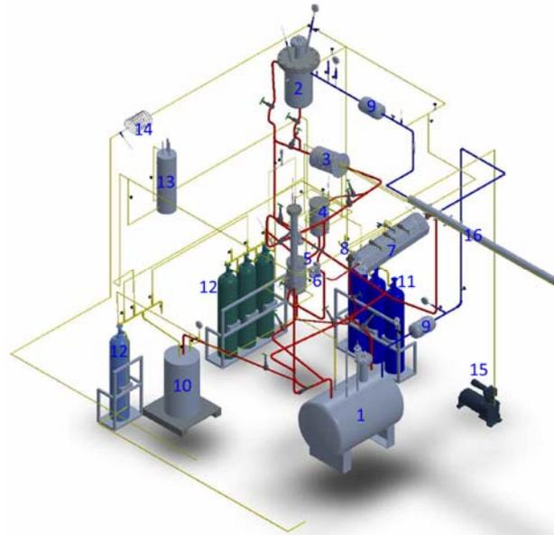
Fig. 1. 3-dimension drawing of the facility (catch tray, electrical heating coils, and insulators are omitted): 1, storage tank; 2, reservoir tank; 3, EMP; 4, coarse filter; 5, fine filter; 6, EMFM; 7, plugging test section; 8, MFC; 9, vapor trap; 10, dump tank; 11, CO<sub>2</sub> cylinder; 12, Ar cylinder; 13, gas heating storage; 14, gas cooler; 15, air compressor; 16, gas collector.
