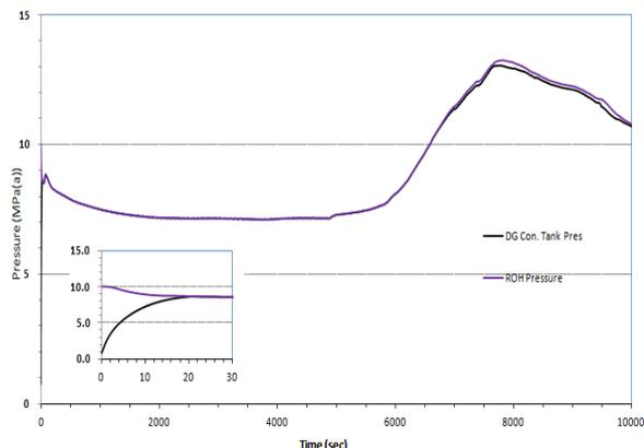
Fig. 3. PHT and DCT pressures of CATHENA(LRV fail open)
