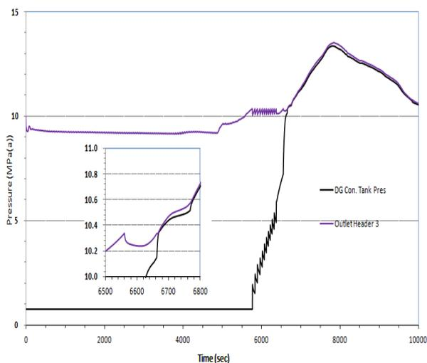
Fig. 2. PHT and DCT pressures of CATHENA(LRV opening at setpoint)
