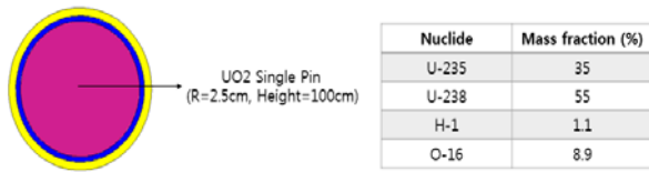
Fig. 1. Structure and composition of the UO2 single pin
