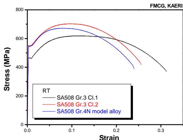
Figure 2 Stress-strain curves of SA508 steels at room temperature
