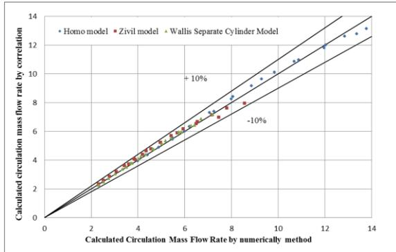
Fig. 6. Error bounds of developed correlations with numerical simulation results
