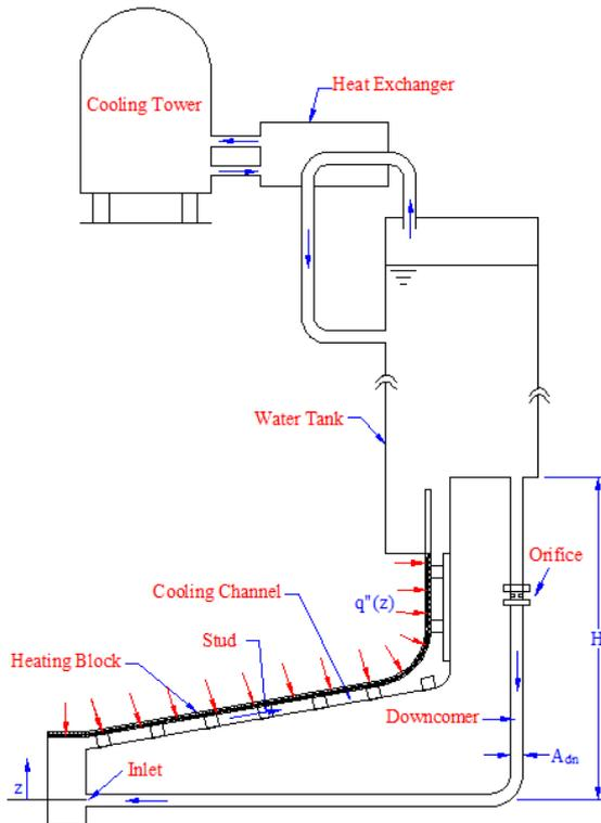
Fig. 2. Schematic of the experimental facility.
