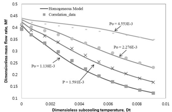
Fig. 5. Variation of the dimensionless mass flow rate along with dimensionless sub-cooling at pressure 1.29 bar (homogeneous model)
