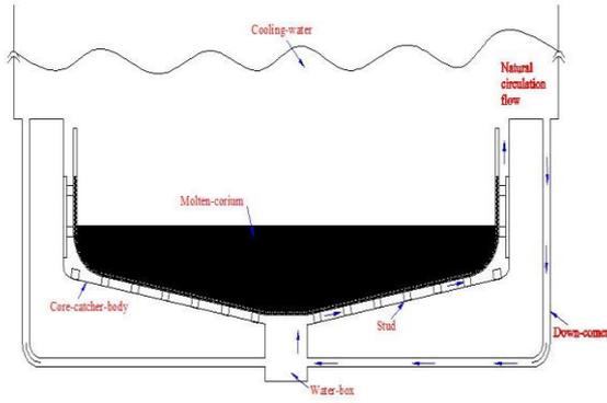
Fig. 1. Schematic of the prototypic core catcher system
