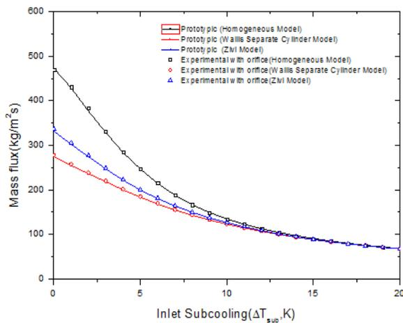
Fig. 3. The calculated mass flux in the experimental facility with an orifice with respect to the inlet subcooling and void fraction model
