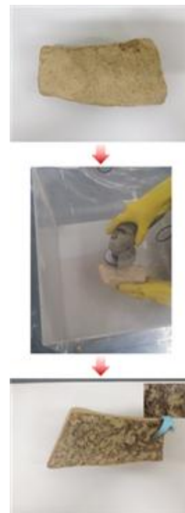
Fig. 1 Decontamination of uranium by grinding method.
