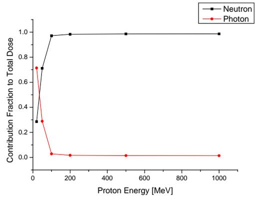
Fig. 3. Dose Contribution Fraction of the Neutron and Photon Generated by Proton Reactions
