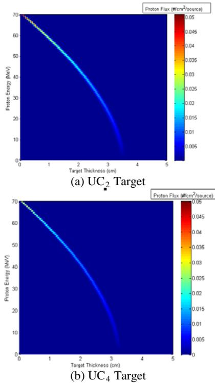
Fig.2. Proton Energy Distribution in the  $UC_2$  and  $UC_4$  Target
