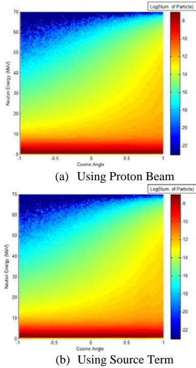
Fig. 5. Angular-energy Distribution of the Neutrons Using Proton-Target Reactions and Source Term for  $UC_2$  Target
