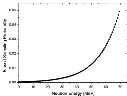
Fig. 10. Biased Source Sampling Probability for the Bulk Shielding Analysis
