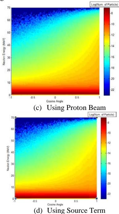
Fig. 6. Angular-energy Distribution of the Neutrons Using Proton-Target Reactions and Source Term for  $UC_4$  Target
