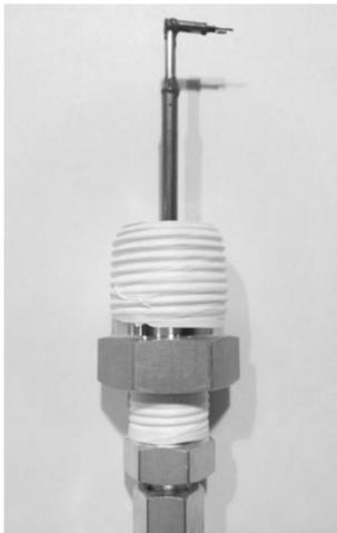
Fig.5. Double sensor conductivity probe
