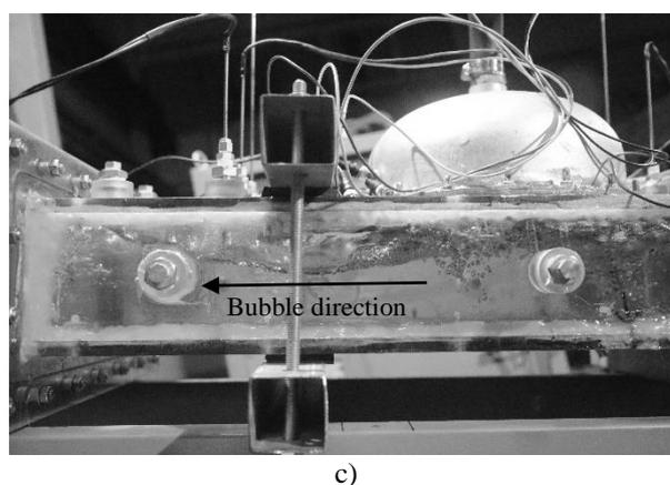
Fig.9. Flow regime in the inclined section: (a) Near the first row of probes; (b) Near the second row; (c) Near the third row
