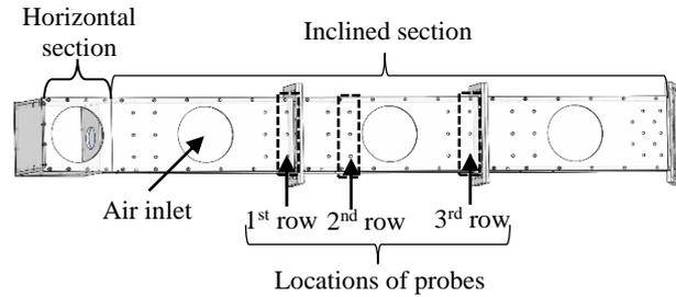
Fig.6. Schematic of the test section and probes' locations in the experiment
