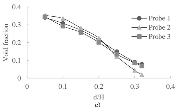
Fig.7. Void fraction profiles at different rows of probes. At each row, probe 1, probe 2 and probe 3 are placed at the same axial location: (a) the first row; (b) the second row; (c) the third row
