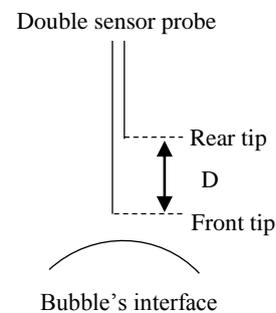
Fig.2. Double sensor probe and bubble's interface
