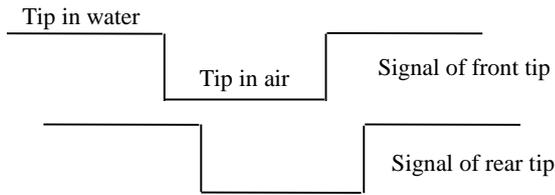
Fig.3. Double sensor probe signal
