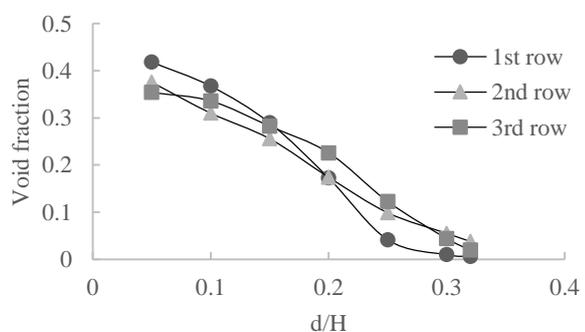
Fig.8. Comparison of void fraction profiles obtained from 3 rows of probes
