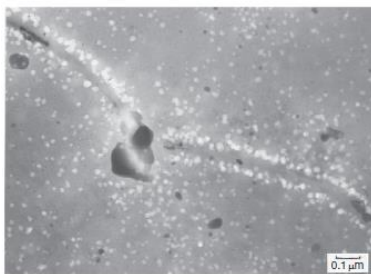
Fig. 2. Denuded grain boundary and associated void enhanced regions in 4-9 purity aluminum after irradiation at 50 °C to a fluence of 3.4 \times 10^{26} \text{ nm}^{-2} ( E > 0.1 \text{ MeV} ) [1].
