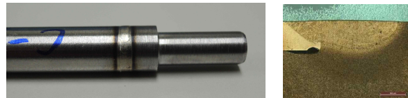
Fig. 6 Weld shape and Microstructure of end plug weld section
