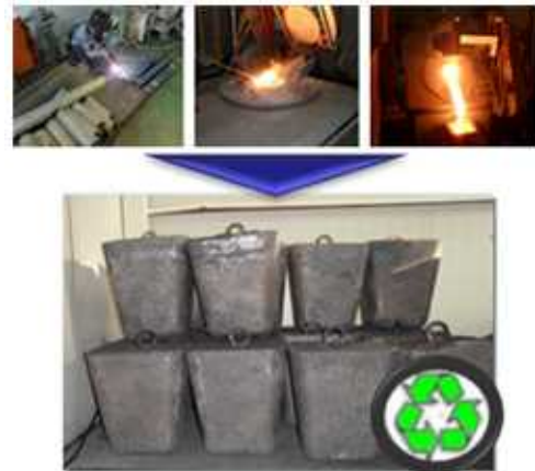
Fig. 3. Melting processing and ingot
