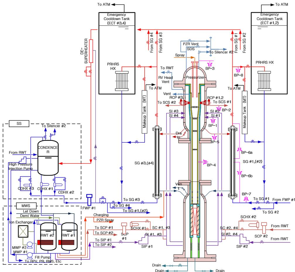
Fig. 1 Schematic diagram of the FESTA facility
