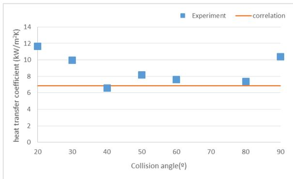
Fig. 7. Heat transfer coefficient versus droplet collision angle
