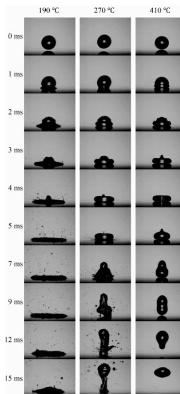
Fig. 1. Droplet collision behavior at 190°C, 270°C and 410°C
