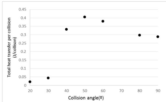
Fig. 3. Droplet collision angle versus Total heat transfer e [3]
