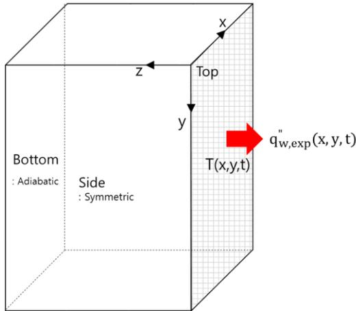
Fig. 6. Setup of Geometry and boundary conditions
