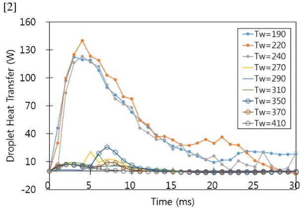
Fig. 2. Droplet collision time versus heat transfer rate [2]
