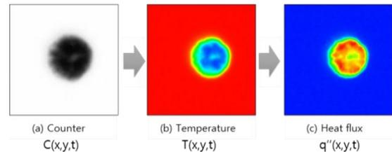
Fig. 5. Calculation procedure for heat flux
