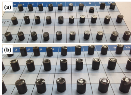
Fig. 6. Impacted pellets having facet surface (a) type P (b) type K of 15^\circ , 45^\circ , 75^\circ respectively in order from up to down.
