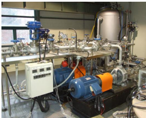
Fig. 1. Flow loop for cavitation experiment
