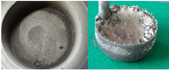
Fig. 3. The re-used graphite crucible coated with TaC/ Y 2 O 3 after injection casting (a), and the residue in the re-used graphite crucible after injection casting (b).
