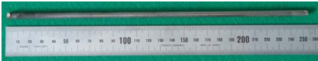
Fig. 4. U-10wt.%Zr-5wt.%RE metallic fuel fabricated by injection casting with the coated graphite crucible.
