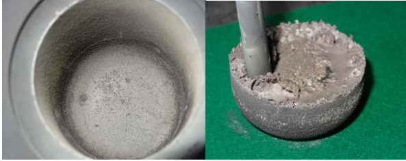
Fig. 2. The TaC/ Y2O3 coated graphite crucible (a), and the residue in the graphite crucible after injection casting (b).
