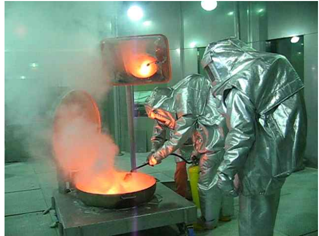
Fig.3. Extinguishment of sodium fire in training cell
