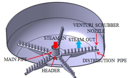
Fig. 3 Geometric depiction of distribution pipe for CFVS
