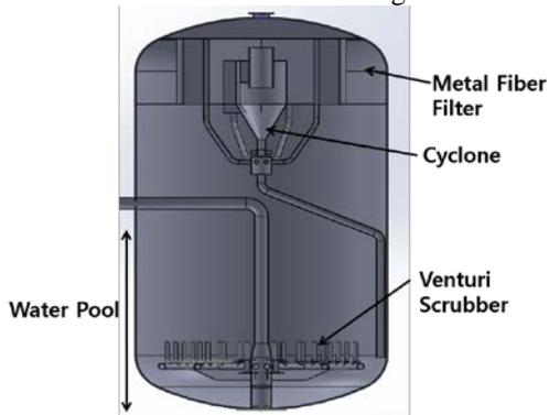
Fig. 1 Containment Filtered Venting System
