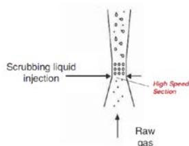
Fig.2 Schematic diagram of venturi scrubber assembly.
