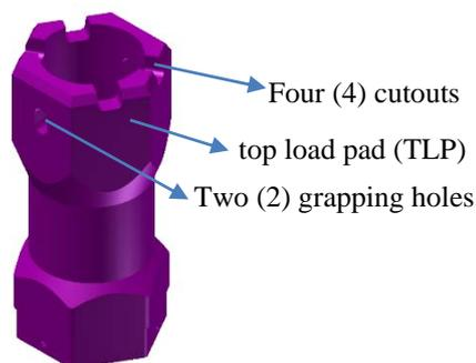
Fig. 3 Schematic drawing of a handling socket.
