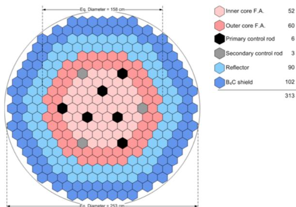
Fig.1 Core radial configuration of 150 MWe for PGSFR.
