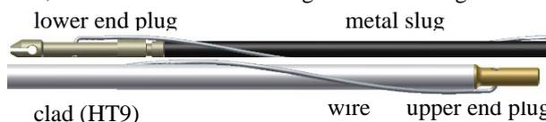
Fig. 7 Detail drawing of a fuel rod for PGSFR.
