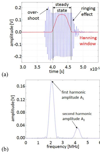
Fig. 2. (a) Time-domain signal; (b) Amplitudes of the first and second harmonics in the frequency-domain, obtained by performing a Fast Fourier transformation on the steady state portion of the time domain signal.
