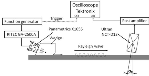
Fig. 1. Schematic diagram of experimental setup using non-contact air-coupled receiver.
