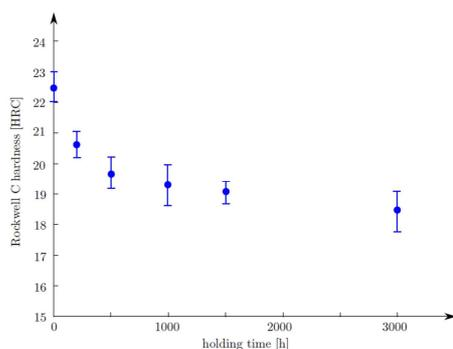
Fig. 6. Rockwell hardness C as function of holding time for mod. 9Cr-1Mo steel.
