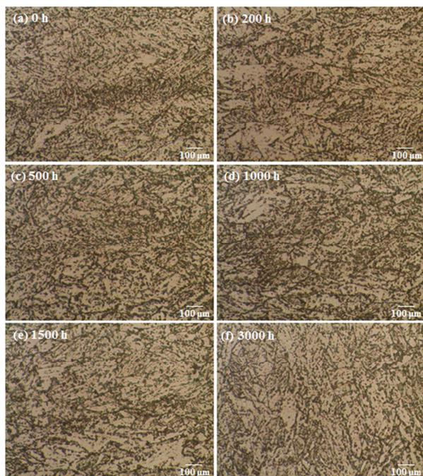
Fig. 5. OM micrographs at 1000X magnifications of modified 9Cr-1Mo steel specimens treated at 650 °C for (a) 0 h (b) 200 h, (c) 500 h, (d) 1000 h, (e) 1500 h and (f) 3000 h
