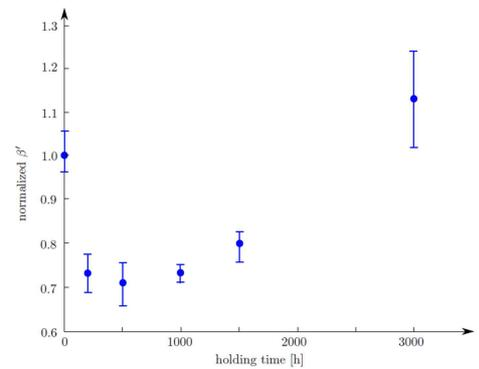
Fig. 4. Nonlinear parameter as function of holding time for 9Cr-1Mo steel.
