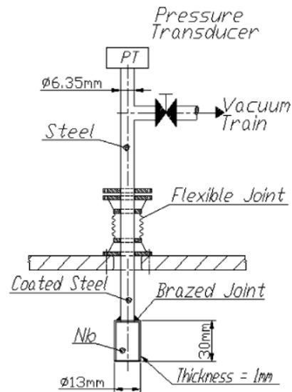
Fig. 1. The Hydrogen permeation sensor design [Ciampichetti et al., 2004, ref. 6]
