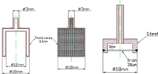
Fig. 3. The optimized permeation sensor designs and its theoretical sensor performance results [Ciampichetti et al., 2007, ref. 7]
