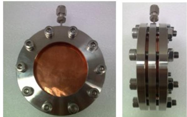
Fig. 5. The flange type permeation sensor with porous structure [Lee et al., 2013, ref. 9]
