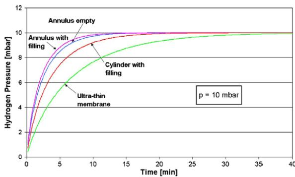
Fig. 4. The optimized permeation sensor designs and its theoretical sensor performance results [Ciampichetti et al., 2007, ref. 7]
