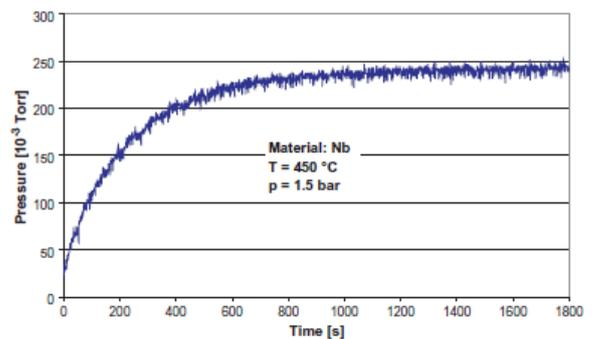
Fig. 2. Performance test result of the permeation sensor [Ciampichetti et al., 2004, ref. 6]
