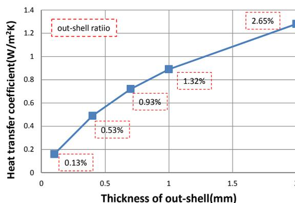
Fig. 4. Heat transfer coefficient of RMI with various out-shell thickness
