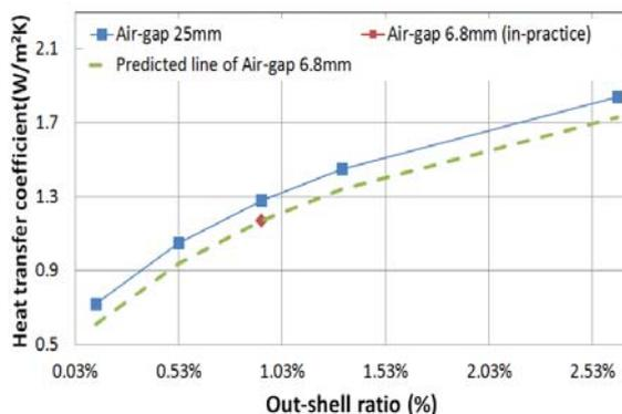
Fig. 6. Prediction of overall heat transfer coefficient for air-gap 6.8mm(in practice) in comparison with air-gap 25mm
