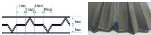
Fig 1. Bending type RMI sheet
