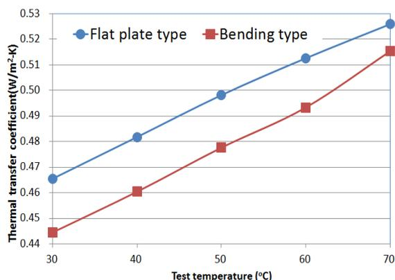
Fig. 3. Heat transfer coefficient of inner-layers for flat and bending type design
