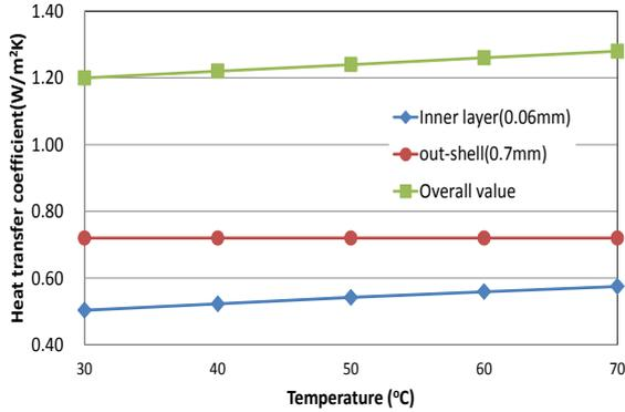
Fig. 5. Sum of heat transfer coefficient of inner-layer and out-shell
