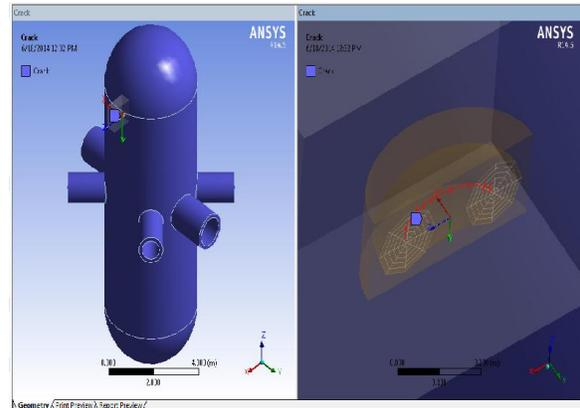
Fig. 8: RPV geometry with crack developed in ANSYS
