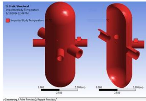
Fig. 15: Steady-state Thermal analysis Body for Static Structural analysis
