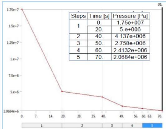
Fig. 12: Pressure profile RPV PTS analysis
