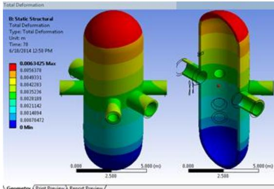
Fig. 16: Total deformation
