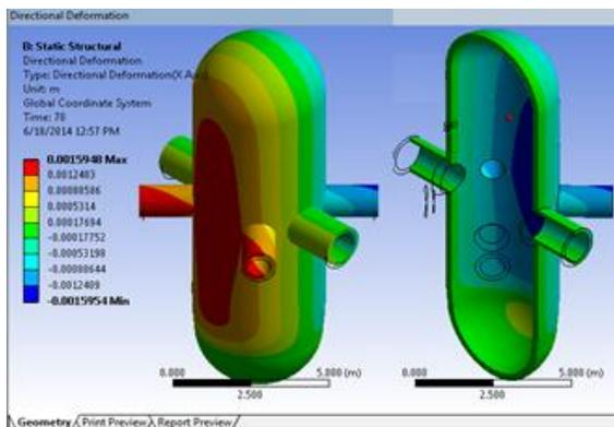
Fig. 18: Directional deformation(x axis)
