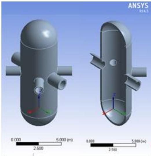
Fig. 7: RPV geometry developed in ANSYS
