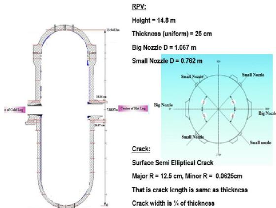
Fig. 6: RPV Simplified Geometry for ANSYS Analysis.
