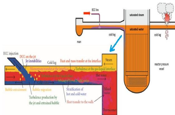
Fig. 1. Simplified PTS event scenario due to LBLOCA in a cold leg of RPV.
