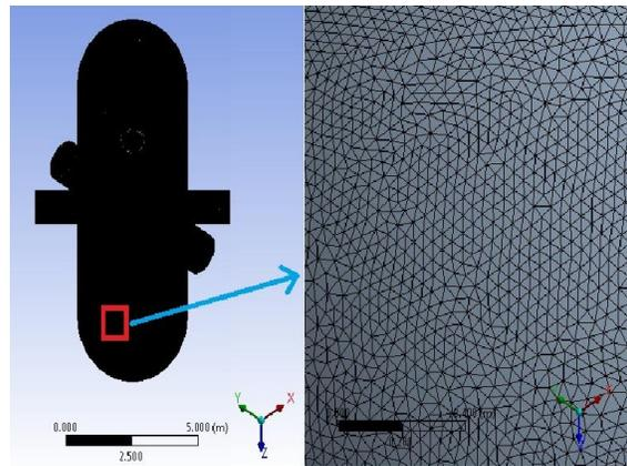
Fig. 9: RPV geometry mesh in ANSYS
