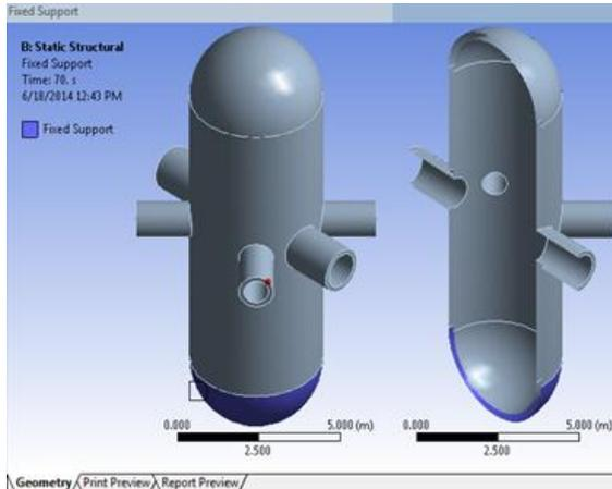
Fig. 10: RPV geometry static structural support in ANSYS
