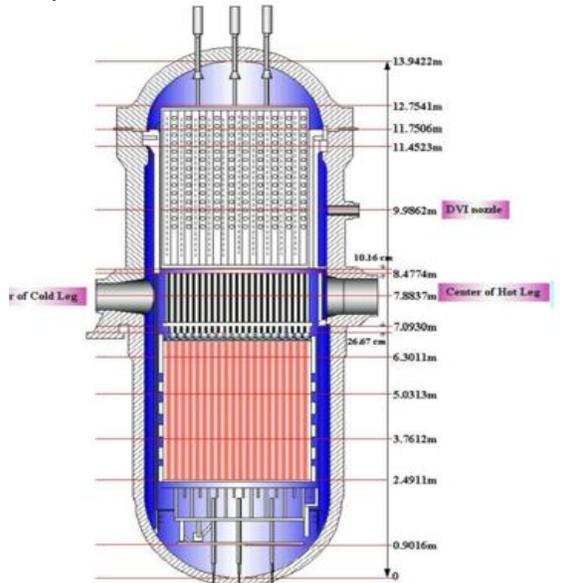
Fig. 5: RPV Original Geometry.
