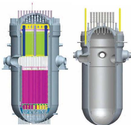
Fig. 2: Reactor Pressure Vessel (RPV) of PWR
