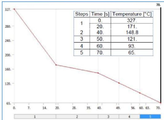
Fig. 11: Temperature profile for RPV PTS analysis
