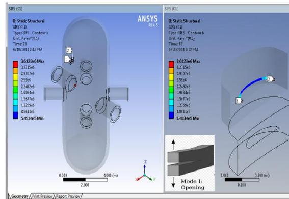
Fig. 21: SIF (Stress Intensity Factor),  $K_1$
