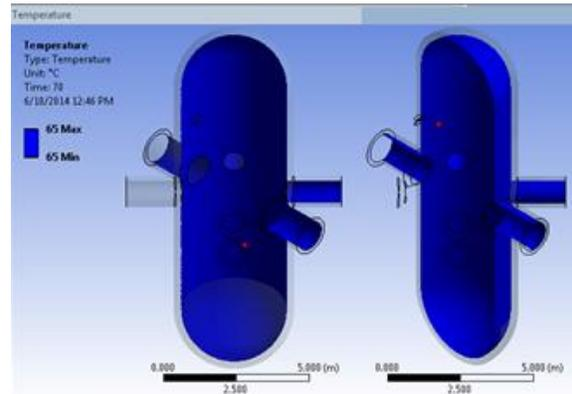
Fig. 14: Steady-state Thermal analysis: Final Temperature
