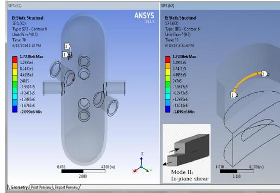
Fig. 22: SIF (Stress Intensity Factor),  $K_2$
