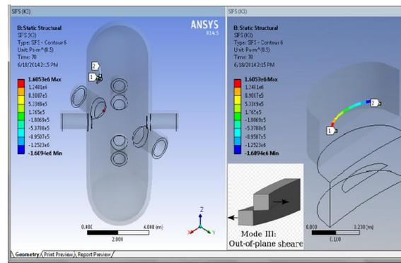
Fig. 23: SIF (Stress Intensity Factor),  $K_3$
