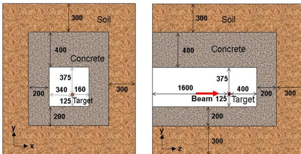
Fig. 2. The configuration of geometry for the calculation of bulk shielding using Monte Carlo code (unit: cm)
