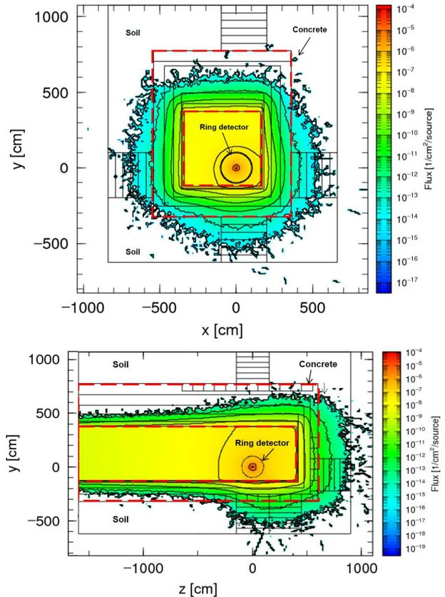
Fig. 3. The secondary neutron distribution of bulk shielding calculation at 90° bending section of RISP using PHITS code.
