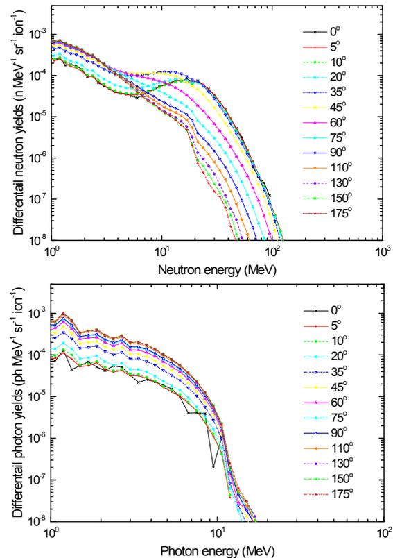
Fig. 1. Differential yields of (a) neutron and (b) photon produced from thick iron target irradiated by 17.5 MeV/nucleon  $^{238}\text{U}$  beams using PHITS code.
