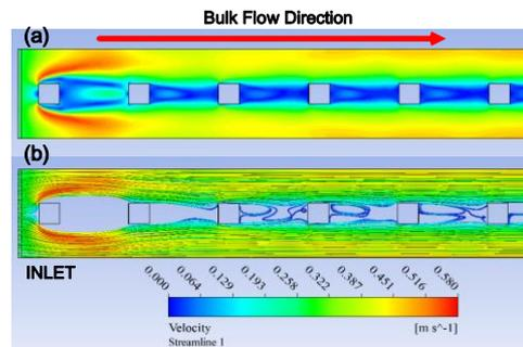
Fig. 9. Calculated flow distribution in the coolant channel containing rectangular shaped studs: (a) contour of velocity magnitude; (b) streamlines
