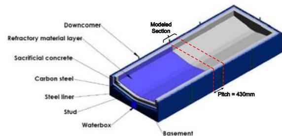
Fig. 5. Schematic diagram of EU-APR1400 Core Catcher [10].
