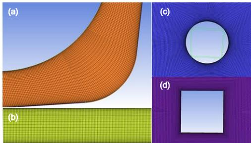
Fig. 7. Generated grids for (a) elbow section; (b) inlet; (c) surrounding of cylinder stud and (d) rectangular stud.
