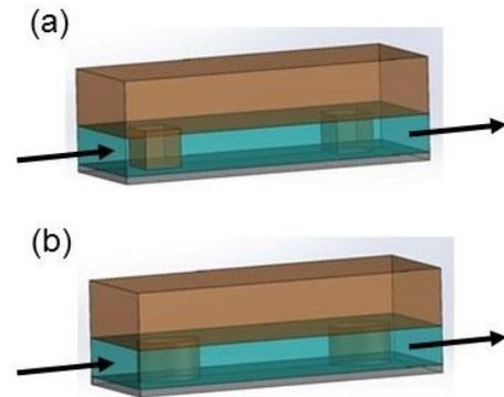
Fig. 4. Suggested examples of the stud shape with the coolant channel: (a) Rectangular stud; (b) Elliptic cylinder stud.
