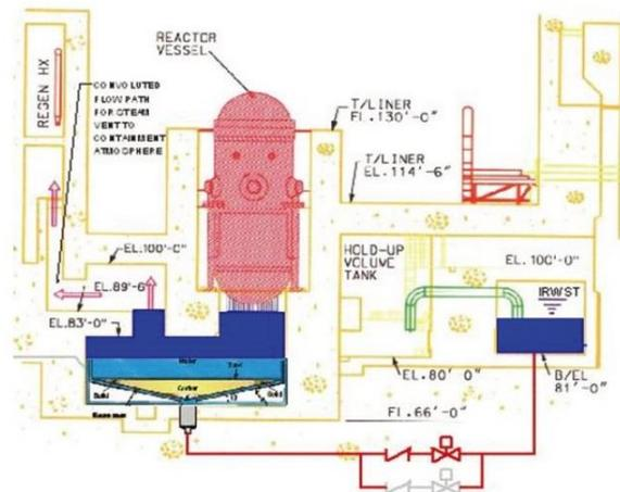
Fig. 1. Arrangement of RPV and ex-vessel core catcher system [4,9].
