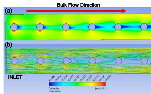
Fig. 8. Calculated flow distribution in the coolant channel containing cylinder shaped studs: (a) contour of velocity magnitude; (b) streamlines
