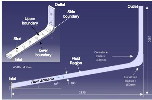
Fig. 6. Schematic diagram of the modeled section in the core catcher.
