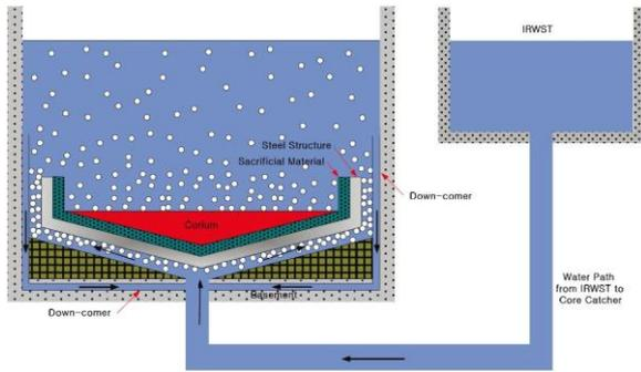
Fig. 2. Conceptual design of the core catcher system with natural circulation [9].
