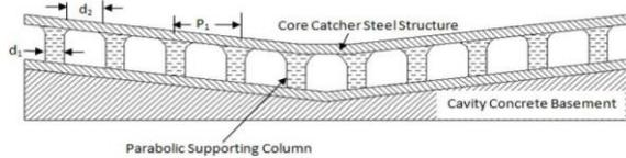
Fig. 3. Side view of the cooling channel [4].
