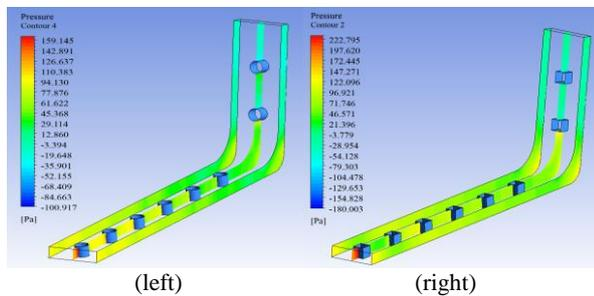
Fig. 10. Pressure contours in the coolant channel containing (Left) cylinder shaped studs; (right) rectangular shaped studs
